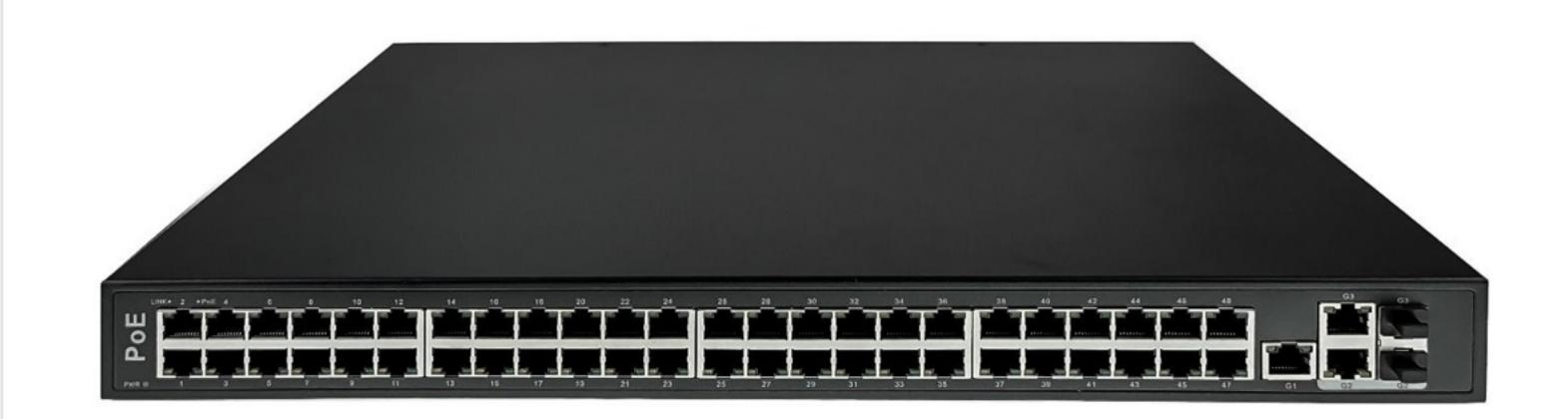
The **IPS-48P2G-AF** is a 48 Port POE Network Switch with 3 Gigabit Uplink Ports | Designed for IP Cameras | POE+ Capable of Pushing 30 Watts per Port | 400 Watts Total Budget
